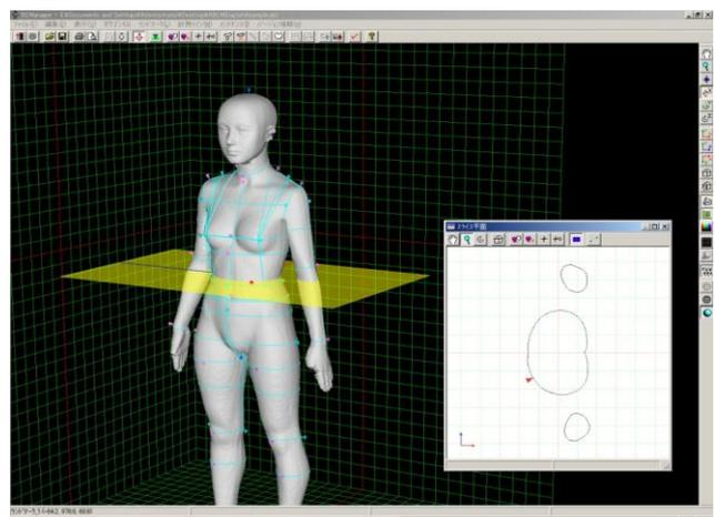
**Figure 1:** Laser beam sheet scanning during human standing posture for determining 3D anthropometric data.
