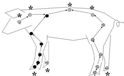
**Figure 1:** Reflective marker model captured with a 3D optoelectronic technique (\* denotes sites where significant movement changes were observed in lame pigs).
