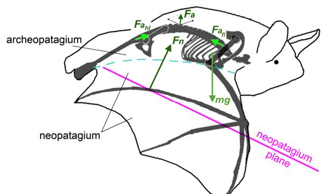
**Figure 1:** Aerodynamic forces applied to archeopatagium and neopatagium in the mid-downstroke.
