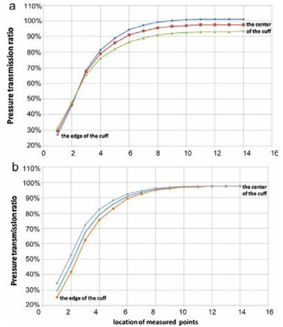
**Figure 4:** FE pressure transmission ratio for soft tissue material properties at CP= 100 mmHg; (a)  $E = 40$  kPa,  $\gamma$ : —  $\gamma = 0.40$ ; —  $\gamma = 0.45$ ; —  $\gamma = 0.49$ . (b)  $\gamma = 0.45$ ,  $E$  (kPa): —  $E = 40$ ; —  $E = 30$ ; —  $E = 60$ .
