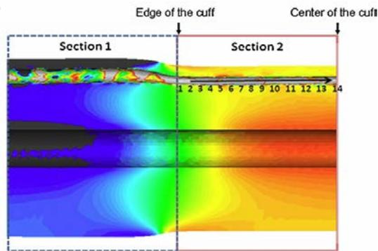
**Figure 3:** Pressure distribution of FE model under cuff pressure in longitudinal direction, when CP = 100 mmHg.
