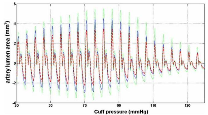
**Figure 5:** FE artery lumen area vs. CP of the mid section predicted: — normal artery; ..... soft artery; --- hard artery.
