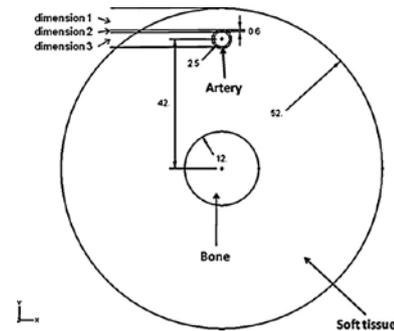
Figure 1: Transverse section of the FE arm model (mm).
