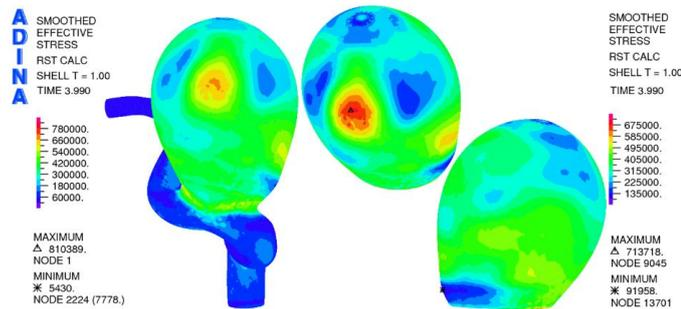
**Figure 1:** Smoothed effective stress on the aneurysm for the systolic time.
