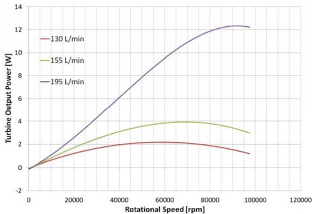
**Figure 2:** Turbine characteristics at different flow rates
