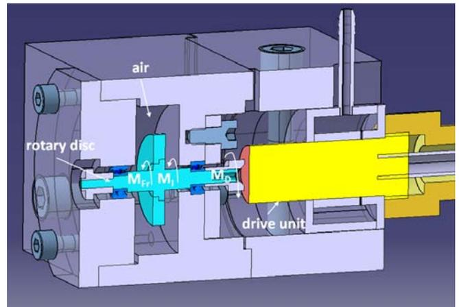
Figure 1: Torque test setup (Viscometer)
