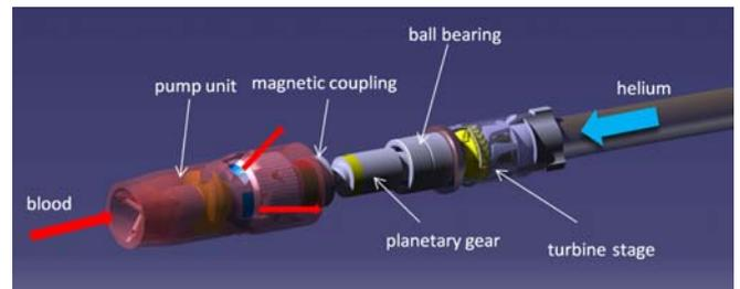
**Figure 3:** Assembly of a heart catheter pump
