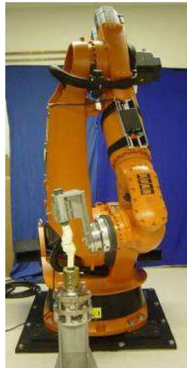
Figure 2: Human knee joint mounted to a serial robot in Dr Woo's laboratory.
