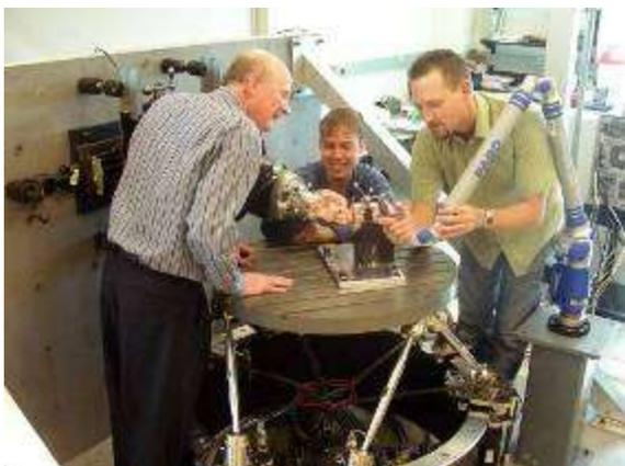
Figure 4: Dr Nigel Shrive, Shon Darcy & Josh Rosvold using a FARO arm to digitize points on a sheep stifle joint (knee) to define the alignment
