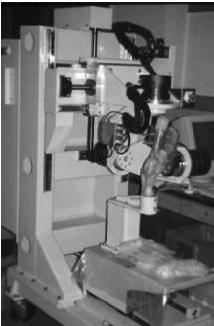
Figure 1: Human knee joint mounted to the robotic joint simulator in Hiromichi Fuji's laboratory at Kogakuin University, Tokyo, Japan.
