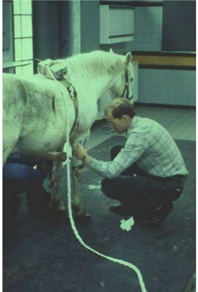
Ton preparing his subject. Note the Kistler charge amplifier on the back. This was needed for the piezoelectric accelerometer that was used as a heelstrike detector
