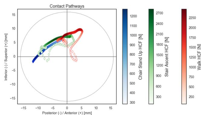
**Fig 2:** Mean resultant hip contact force pathways for gait, stair ascent and standing up from a chair.
