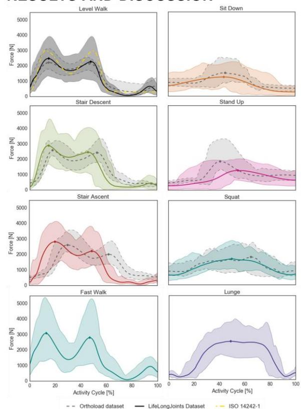
**Fig 1:** Predicted mean HCF, with min/max range of variation, across 132 patients for different ADLs, compared to data from instrumented implants [1] and current preclinical testing standards.
