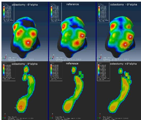
Fig 1: Stress over talar (above view) & plantar pressure
