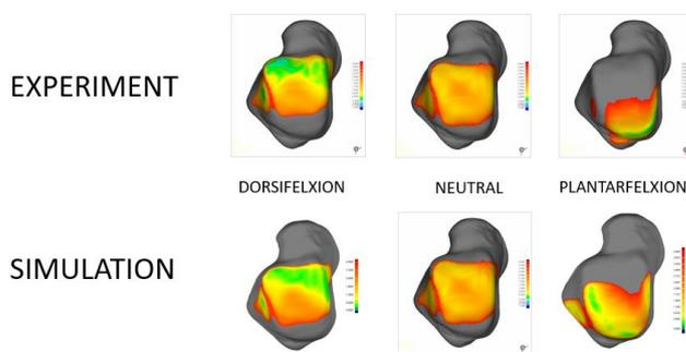
Figure 6 – Comparison of distance maps at the ankle joint in neutral and in extreme dorsiflexion and plantarflexion position, between the experimental data and the results of the simulation for one specimen.
