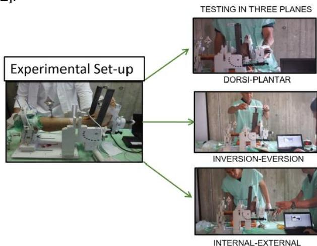
Figure 1 – Experimental set-up for testing the cadaver legs in three planes. The applied torque and the displacement of hindfoot bones (calcaneus, talus, tibia) were recorded.
