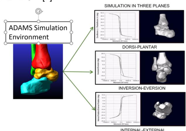
Figure 3 – ADAMS simulation environment for simulating Ankle behaviour in three planes.
