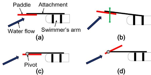
**Fig 2:** Schematic figures explaining the improvement of paddle. (a) The water flow comes from the front when gliding. (b) Instability to turn over the paddle occurs. (c) New structure with a pivot. (d) The paddle can rotate so that the instability does not occur.
