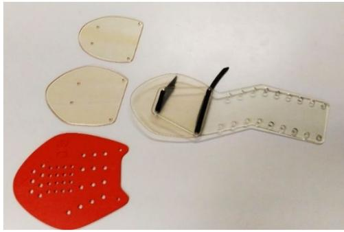
**Fig 1:** Initially developed paddle. The plate on the right is an attachment between the arm and paddle. The swimmer could choose the large (on the top left) or small (on the middle left) paddle. The bottom left is a paddle on the market.
