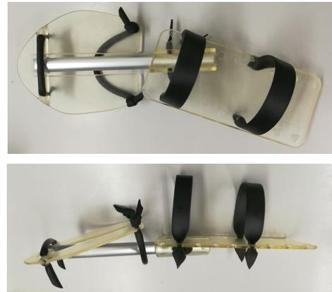
**Fig 3:** Finally developed paddle. The rubber tubes on the paddle prevent excessive rotation of the paddle. The rubber bands on the attachment are for the fixation to the swimmer's arm.
