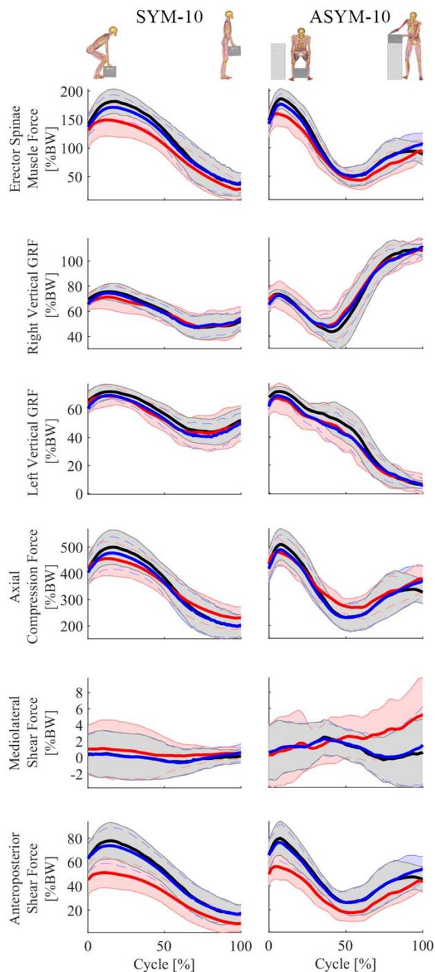
**Fig 1:** Mean forces (solid line)  $\pm$  1 SD (shaded area) for the OMC-MGRF (blue), OMC-PGRF (black) and IMC-PGRF (red) models during SYM and ASYM of a 10 kg box.
