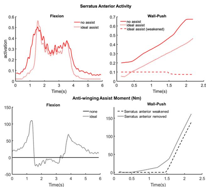
**Fig 3:** The effect of ideal anti-winging assist on SA activation during flexion with 2kg weight and wall-push tasks (top row). Ideal assist moments applied during flexion and wall-push (bottom row).
